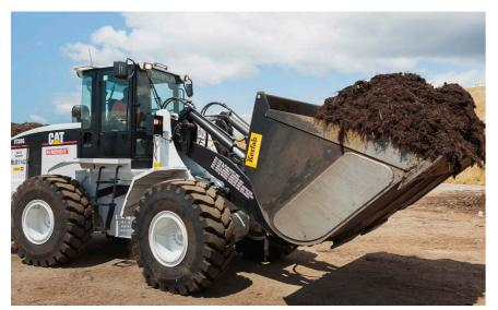
People often want the largest bucket their machine can handle, but the materials being handled dictates the style and size of the required bucket. Dense and abrasive materials require heavier duty buckets which can weigh considerably more than their lighter duty counterparts.
